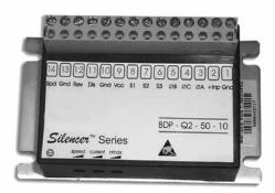
Silencer® brushless controllers are available in a variety of voltage and current ratings. Their compact packaging minimizes space demands. All controllers have generous terminal blocks to facilitate ease of wiring.
