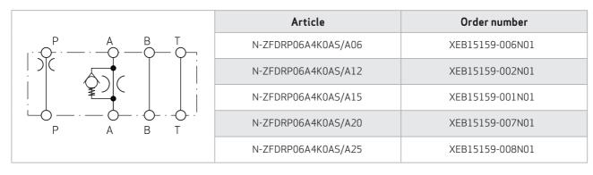
The opening pressure is 0.3 bar, Axx represents the orifice diameter (xx) in tenths of mm in the A port. (Example: ZFDRP06A4K0AS/A25  $\rightarrow$  2.5 mm orifice in A)
