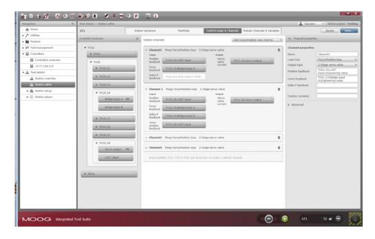
This is the central place to configure the station hardware and software. The user adds specific hardware I/O, creates logical channels and desired control loops, and can add psuedo channels for calculations.
