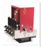
The Moog Hydraulic Service Manifold (HSM) provides on/off hydraulic pressure with an adjustable transition from off to high pressure. Filters protect sensitive servo valves and accumulators provide instantaneous flow or pressure damping when needed. Several flow-rating sizes with 1 to 4 station options are available.
