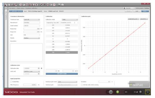
This area allows the user to convert sensor signals (voltages) into desired engineering units. A calibration wizard guides the user through the process in a simple way. Sensor sensitivity can be directly entered or calculated from up to 99 points for precise linearity.
