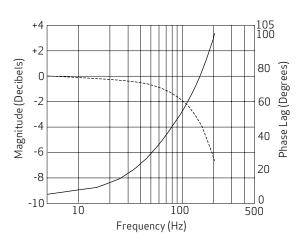
Measured with 40 % signal amplitude, at 3,000 psi (210 bar) pilot or operating pressure, fluid viscosity of 24 cSt, and fluid temperature of 104 °F (40 °C)
