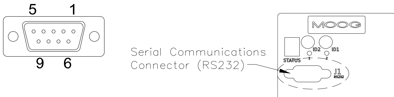
Figure 3-50 RS232 Connector Locations and Pinout
