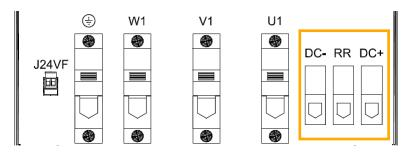
Figure 22: Connector [DC- RR DC+] sizes L355
