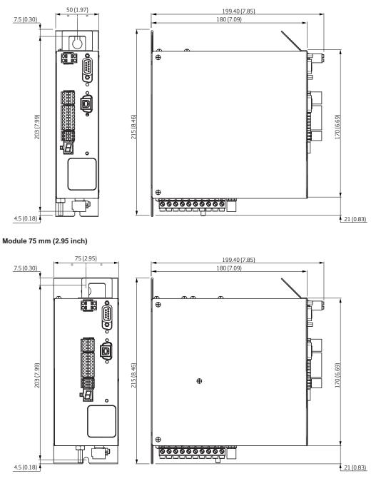
Figure 5: Drive Chassis Dimensions (L50 and L75)
