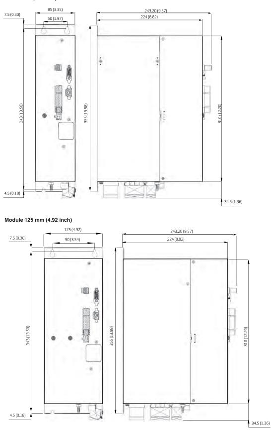
Figure 6: Drive Chassis Dimensions (L85 and L125)
