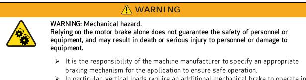
In particular, vertical loads require an additional mechanical brake to operate in a certifiably safe manner.
