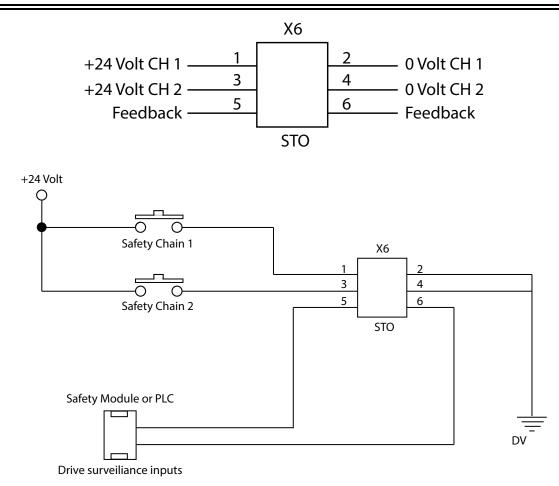
Figure 27: Detail of the Feedback Contact Circuit
