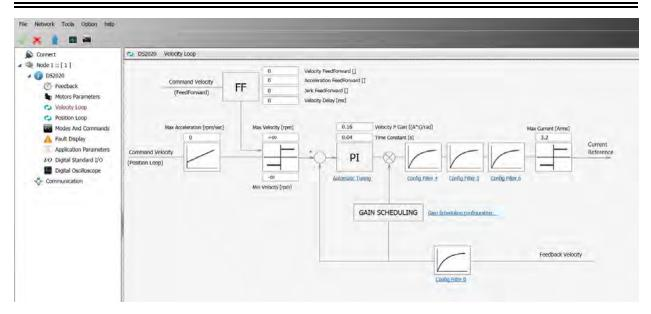
A standard correcting block (PI in the above image) is characterized by two parameters. It is followed by a sequence of filters, and a filter on the feedback chain. This allows the implementation of more complex control structures as well as filtering of known disturbances (Notch filter).
