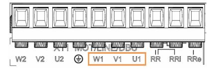
Figure 18: Connector X11 – [W1-V1-U1] sizes L50 and L75
