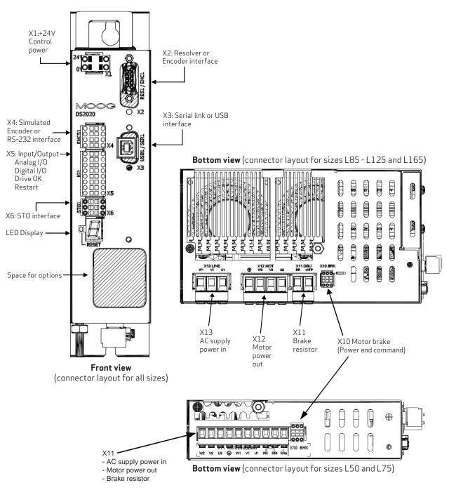
Figure 8: Drive Front Panel and Bottom Connectors
