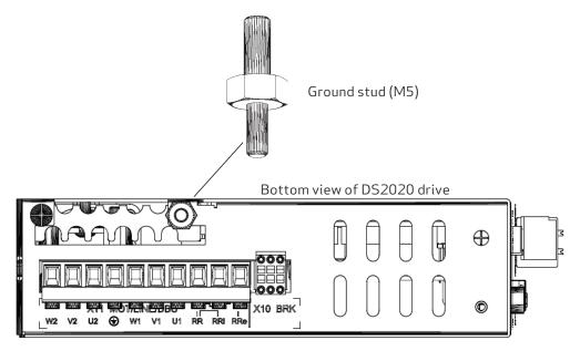
Figure 16: Location of the Ground Stud (M5)
