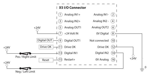
Figure 32: Example I/O Connections on the X5 Connector
