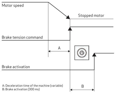
Figure 26: Brake Activation Timing Diagram
