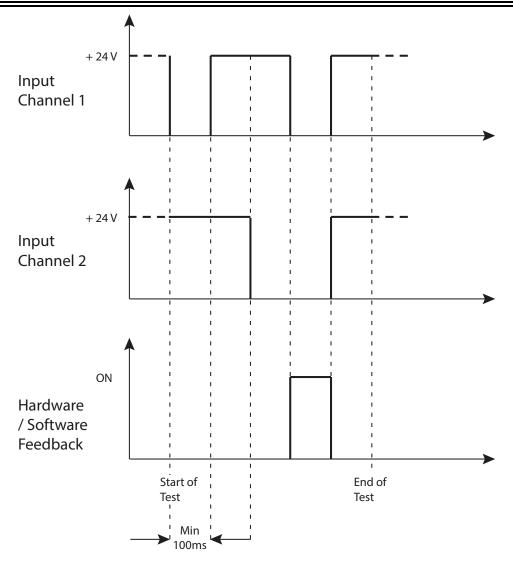
Figure 31: STO Mandatory Sequence Circuit Test
