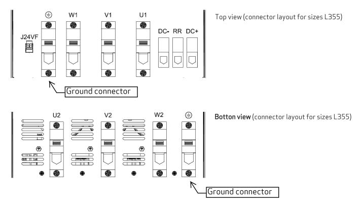
Figure 17: Location of the Ground Connector size L355
