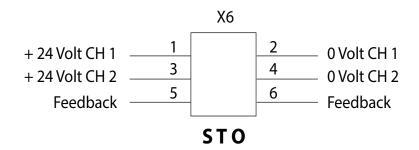
Figure 29: Movable Connector Pinout: 6 Contacts, Model B2 3.50 / 06/180 SN BK BX Weidmuller
