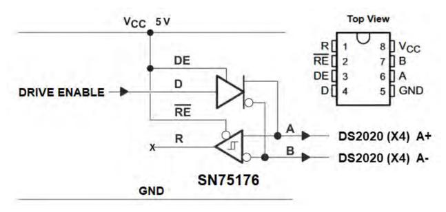
Figure 33: Example RS-485 Driver Using the SN75176 IC
