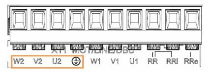
Figure 23: Connector X11 - [W2-V2-U2-] Sizes L50 and L75
