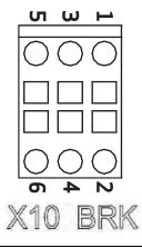
The brake control circuit must be externally powered through X10.
