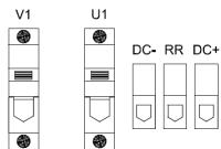
Top view (connector layout for sizes L355)
