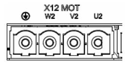
Figure 24: Connector X12- [W2-V2-U2-] Sizes L85 and L125
