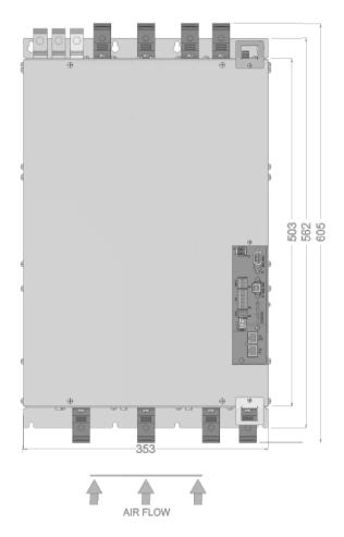
Bottom view (connector layout for sizes L355)
