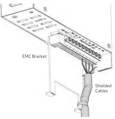
Figure 15: Connection Cables EMC Bracket on size 50 mm
