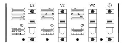
Botton view (connector layout for sizes L355)
