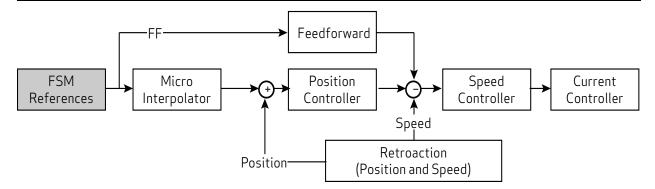
Depending on the structure chosen, the reference for torque, speed or position must be provided.
