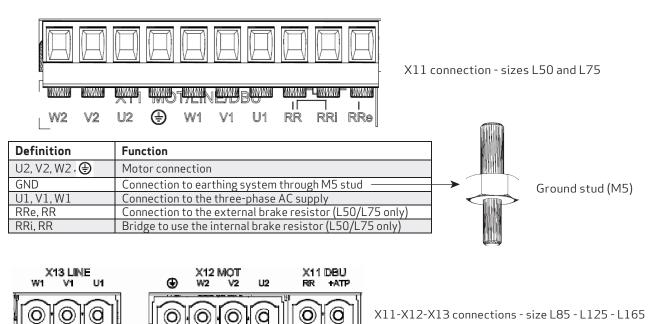
The cable must be shielded. The shield connection to ground can be closed with a conductive strap, which is used to connect the cable to the metal bracket fixed under the drive.
