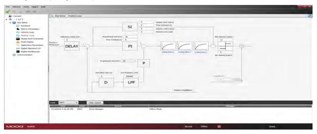
It recognizes the standard control loop (PID) characterized by four parameters. That is followed by a sequence of filters that the implementation of more complex control structures. For parameterization of the filters, see Filter configuration on page 103.
