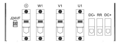
Top view (connector layout for sizes L355)
