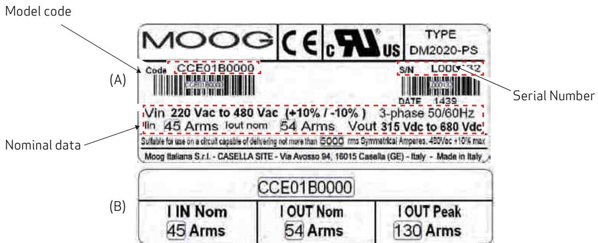
Example of power supply side plate (A) and front plate (B)
