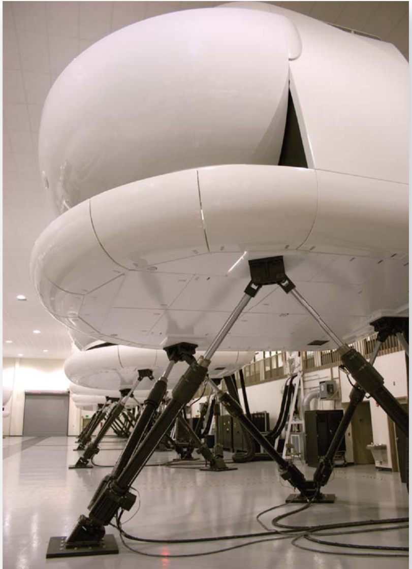
The underside of a FlightSafety International full-flight simulator shows the six electric linear actuators that move the “cockpit” of the simulator to replicate the flying parameters of various aircraft. The hexapod arrangement lets the cockpit travel through six degrees-of-freedom (6DOF) .
