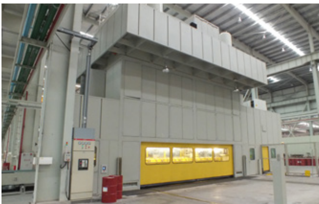
All images and drawings are the property of Moog. A Chinese Tier 1 supplier is using a transfer press for the manufacture of body parts for the auto industry. Moog provided a controlled two-point die cushion system for precise and highly efficient part production.
